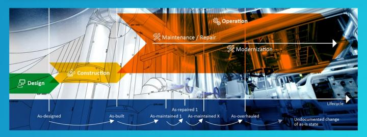
The first differences between the design of a plant (as-designed) and the plant that is actually built (as-built) can be seen as early as the construction phase. Even if these differences are not crucial to the operation of a plant, it means that the as-is documentation is not up to date. In addition, maintenance, repair and modernization activities lead to ongoing changes throughout its lifecycle. Documentation of the as-is state is often neglected.
